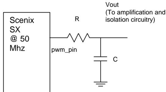
Depending on the maximum frequency you wish to obtain, you should adjust the component values for R and C to choose the resolution of the PWM. Ideally, you should calculate the maximum SIN frequency output you will use and choose the cutoff to be at this frequency. Since the maximum frequency used by the modem software is 2.1kHz, calculate R and C:
