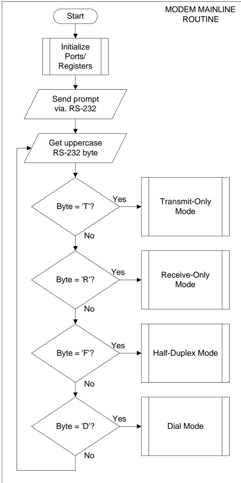
The software consists of an interrupt service routine and a mainline routine. The two routines run independently, with the interrupt service routine running all of the timing sensitive portions of the program, such as the UARTs, timers, A/Ds, D/As, frequency generation, and frequency detection. The mainline routine coordinates, enables, and disables the Virtual Peripherals when necessary to create the overall modem algorithm.
