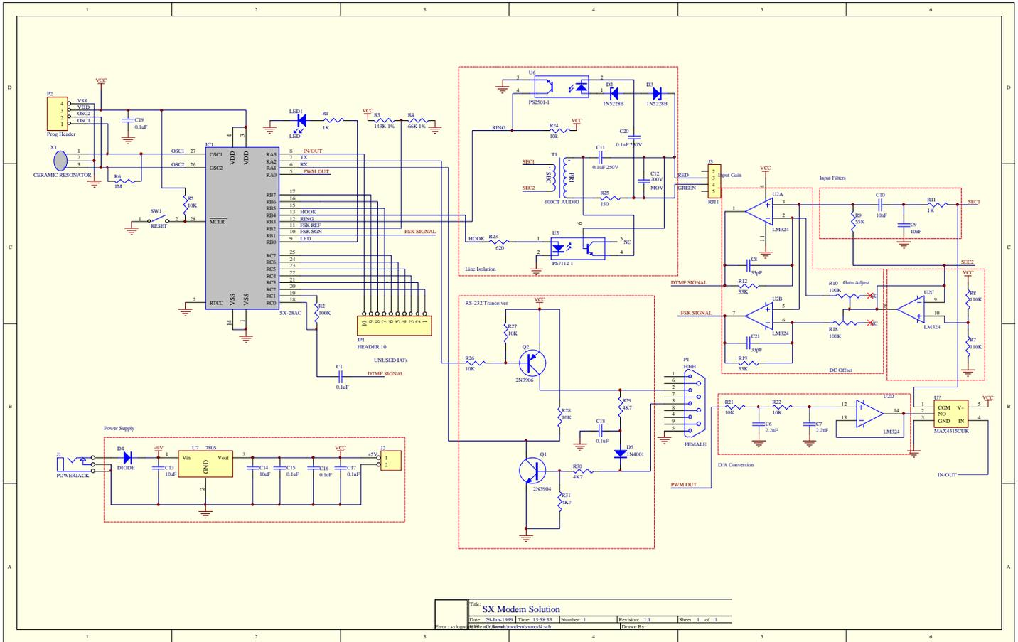
This schematic shows the latest revision of the hardware. Since the design of this board, we have found that much of the hardware is unnecessary, such as the potentiometers, the analog switch, the comparator reference resistors, and, quite possibly, the op-amp. Keep in touch with [www.scenix.com](http://www.scenix.com) for any updates we make available.
