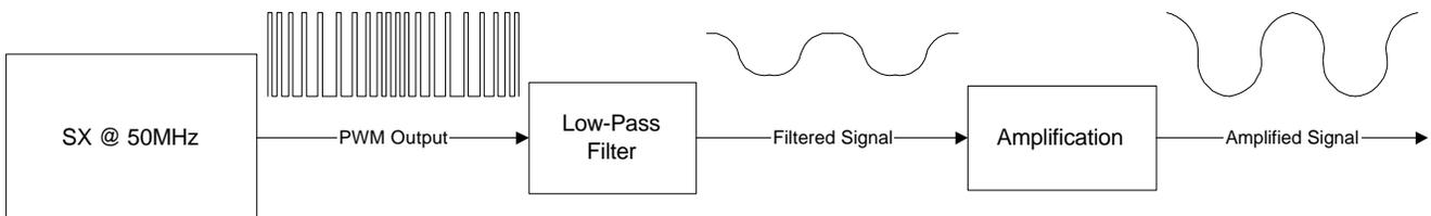
To convert the internal digital values inside the SX back into real-world analogue signals, a Digital-to-Analogue converter (D/A) is required. The SX modem uses a single 8-bit PWM virtual peripheral to accomplish the conversion. A PWM register is loaded with a value from 0 to 255, and this value represents the duty cycle of the PWM output. For DTMF generation, the PWM register is loaded with the sum of the amplitudes of each of the sine waves representing the digit.
